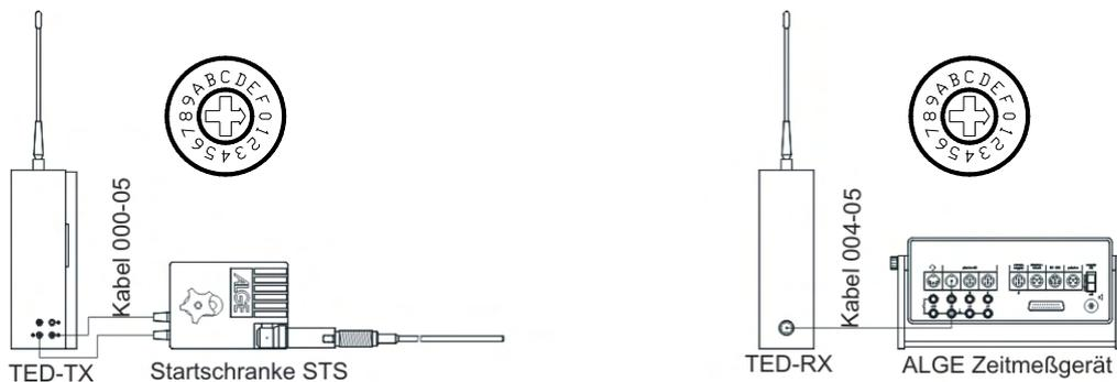
TED –TX and RX must be adjusted to the same address.
