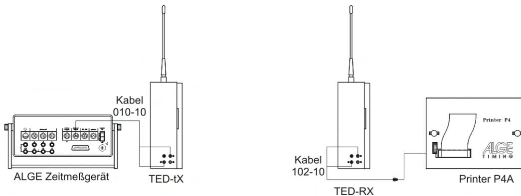
If the output „RS232“ is used by a timing device, you must use cable 060-10 for the TED-TX.
