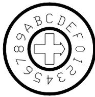
Chose the requested address with the provided screw driver. The arrow of the switcher shows the position. Our factory settings is at position 0.
