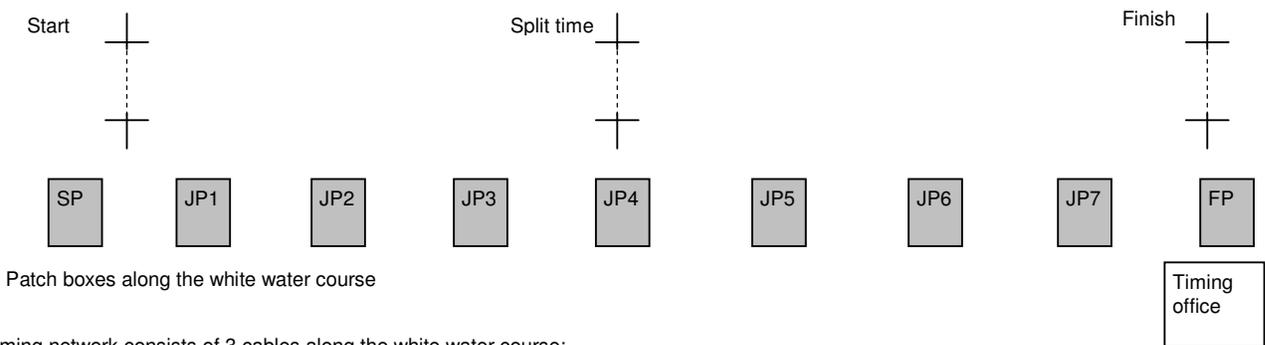
The timing network consists of 3 cables along the white water course:
