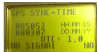
When “OK -UTC +UTC NO” is displayed in the bottom line, the time for your region can be adjusted with keys <F1> and <F2>. As soon as the correct time is shown, press <OK>.
